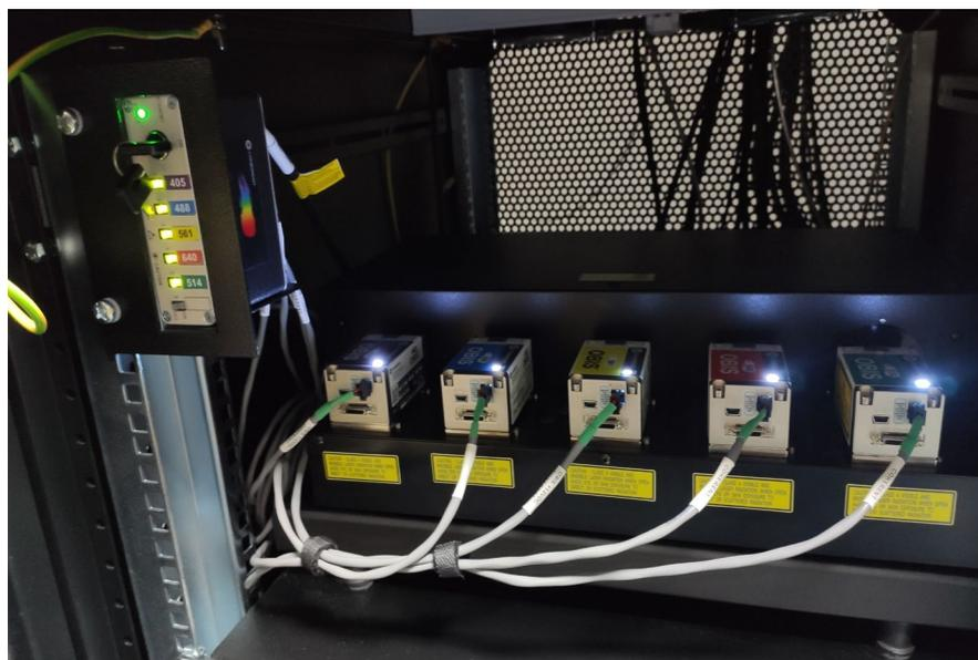
9- Detectores Multi Alkali PMT (SD) y GaAsP PMT (HDS).
